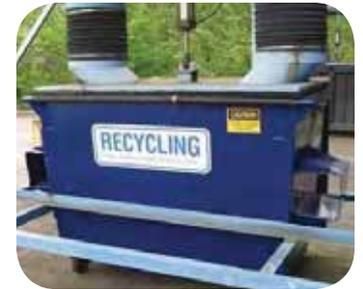
*“Cyclone waste” (i.e., lighter weight material such as paper transfers and plastic bottles) is collected for recycling by a vacuum system used to clean buses at transit bases.*
