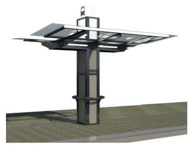
Canopy Type #5 Mini-Canopy is 15-0" long with glazing panels on the both sides of the roof and two real time arrival screens within the pylon.
